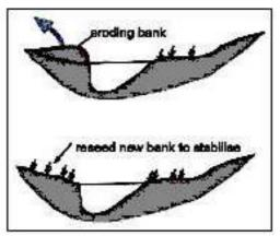
Fig. 4.3. Compound channel (left) and bank re-shaping (right) (based on WWF 2002).
