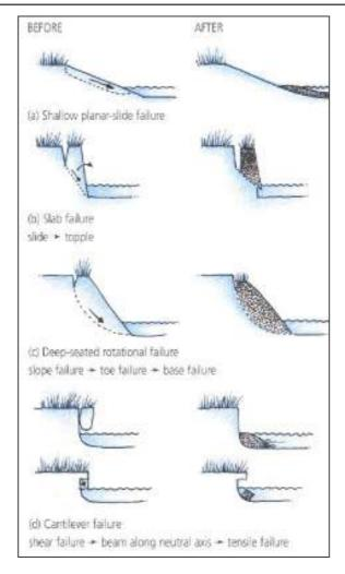
Fig. 4.2. Types of mass failure of river banks (based on Hemphill and Bramley (1989) in Rutherfurd et al. (1999).
